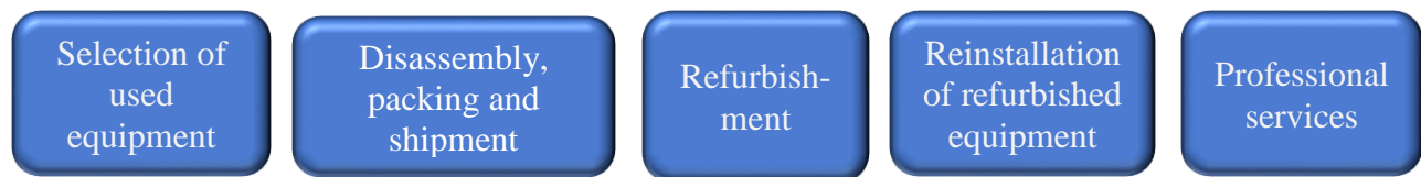
Figure 1. Recommended steps for refurbishing process
