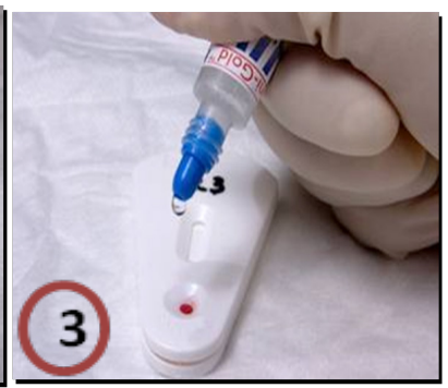
3 Add 2 drops (approx. 60µl) of the wash reagent to sample port
