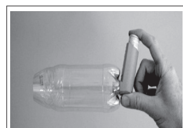
Figure 47 Locally made spacer from plastic material
